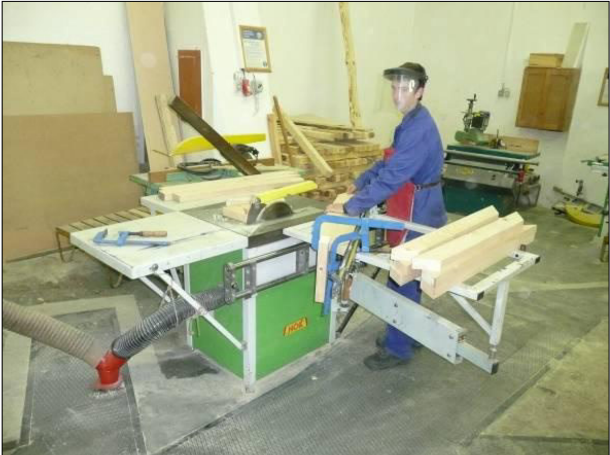
Figure 6 Cutting of the timber material
