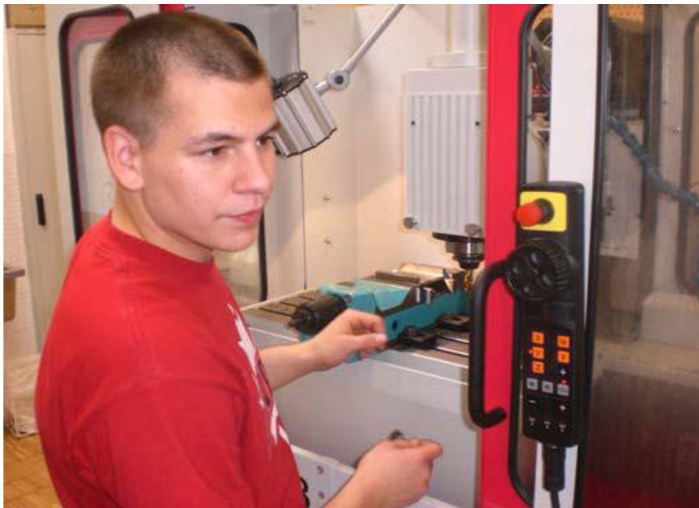
Figure 2: Milling the stamp-fastening plate.
